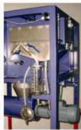
HDR dosage system
