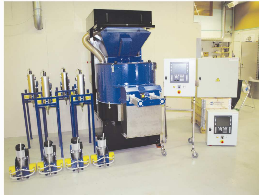
The picture shows a standard equipped R1000 batch treater equipped with 4 dosage systems for liquids and 2 control cabinets
